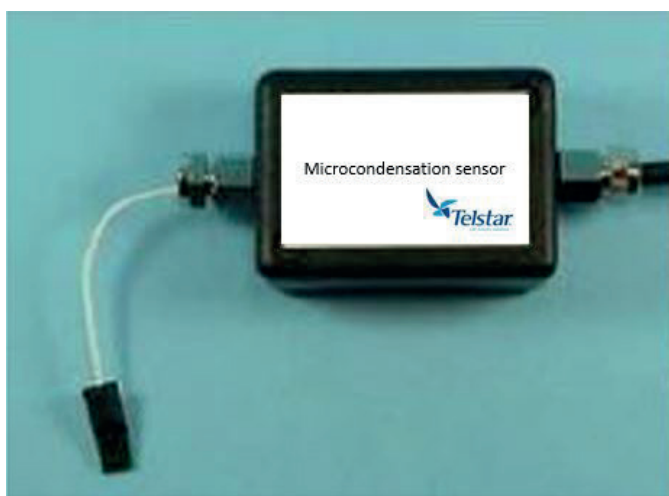
Figure 1: Micro-condensation sensor used to measure the impact of liquid hydrogen peroxide
