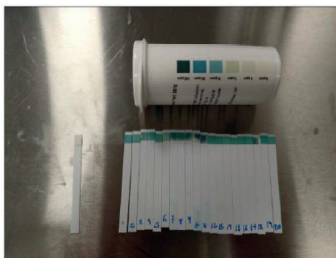
Figure 3: Chemical indicators after being exposed to a hydrogen peroxide cycle
